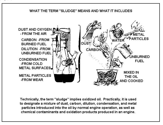
Figure 3-3. Engine sludge
