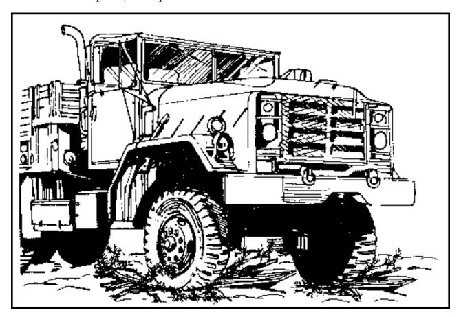
Figure 3-2. Place material under tires to prevent freezing
