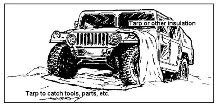
Figure 1-4. Tarps used to protect from cold and to catch dropped parts
