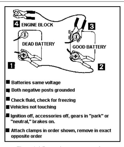
Figure 1-6. Proper jump-start procedure
