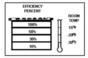
Figure 1-5. Battery efficiency at varying temperatures
