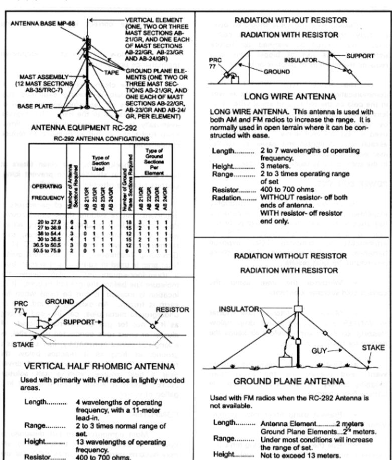
Figure 6-1. Antenna dimensions
