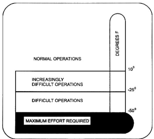
Figure 1-1. Operational difficulty vs temperature range
