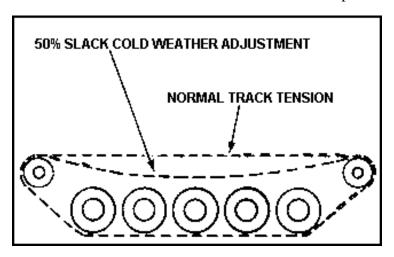
Figure 2-1. Cold weather adjustment
