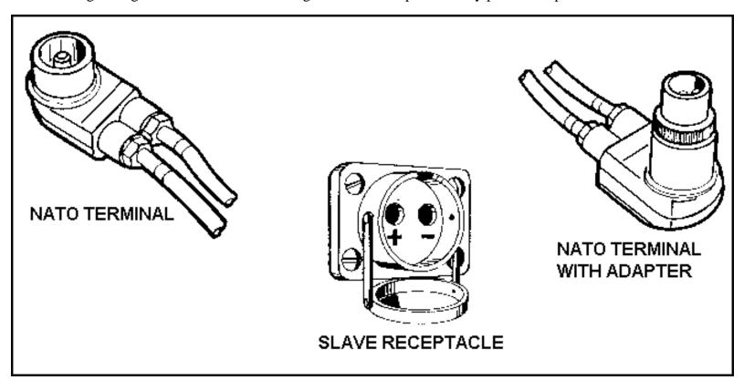
Figure 1-8. Auxiliary power (slave) receptacle and terminals
