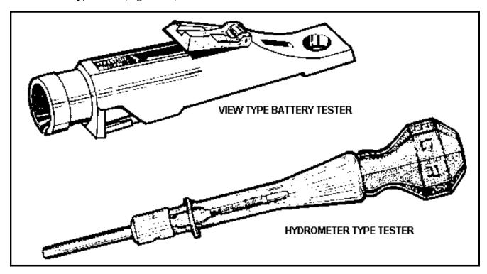
Figure 2-2. Antifreeze testing devices
