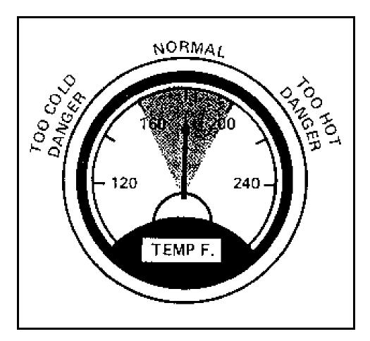
Figure 3-5. Normal operating temperature
