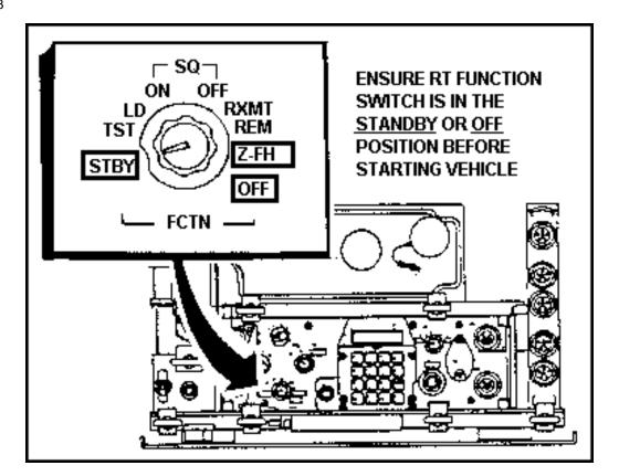
Figure 3-1. Protect radios when starting vehicles
