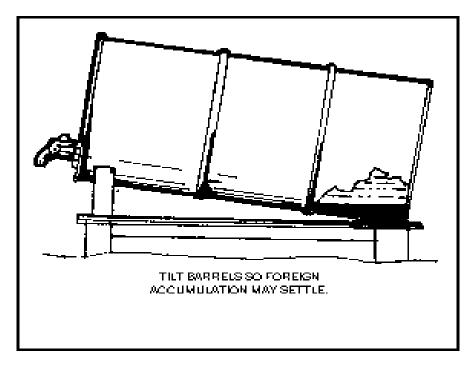
Figure 3-4. POL barrel storage
